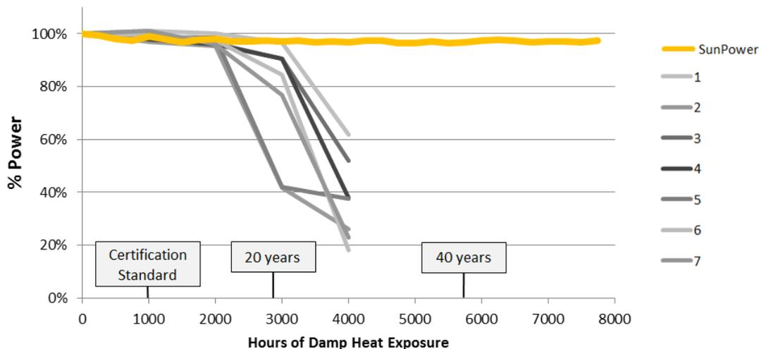
**Figure 1: Damp heat testing of seven Conventional and SunPower modules. The Conventional Modules in Köhl's study show a sharp power drop starting after 2000 hours, while SunPower modules remain relatively unaffected beyond 7000 hours. Equivalent years in a hot and humid environment (e.g. Bangkok) [2] are shown on bottom axis. Sensitivity analysis gives  $\pm 30\%$  on 20 year equivalent time.**
