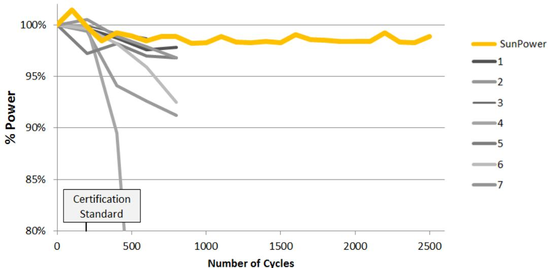
**Figure 2: Thermal cycle testing of seven Conventional and SunPower Modules. The Conventional Modules in Köhl's study start to degrade steadily after 200 cycles, while SunPower remains practically unaffected at 2500 cycles.**
