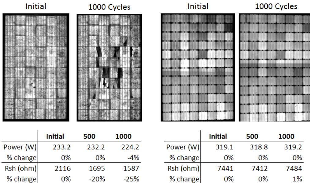
**Figure 3: Electroluminescent images flash test data after 1000 cycles of dynamic loading to 2400Pa (equivalent to 130mph (209kph) wind), conducted at SunPower. The Conventional Module (left) suffered from power loss while the SunPower module (right) was not significantly affected.**
