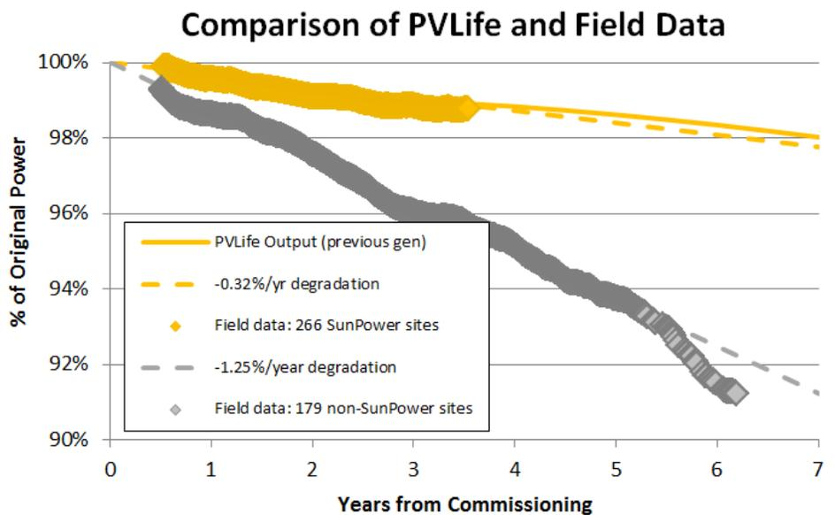
**Figure 7: Comparison of PVLife and analyzed field data from the previous generation of SunPower modules (yellow). PVLife compares well with field data. For reference, the degradation of Conventional Modules is included (grey).**
